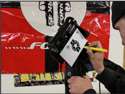
Install template to frame. Trace along the edge of the template to create a guide line for cutting.
