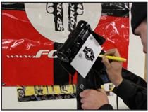
Install template to frame. Trace along the edge of the template to create a guide line for cutting.
