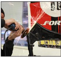
Bevel edge of neck and deburr for a clean weld.
