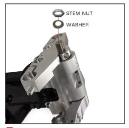
5 Install top tree on stem. Next place a washer on to the neck stem, then add 1 stem nut. Torque top stem nut until bearings feel seated 30ft lbs. - DO NOT tighten stem pinch bolt at this time
