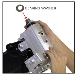
4 Install second bearing over tree stem, (be sure to grease the bearing) then place washer on top of the bearing.
