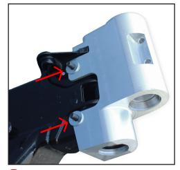
3 Install the two washers on the opsite side of bolt on neck.
