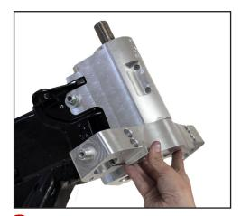
3 Insert lower tree stem through the bottom of the steering tube.
