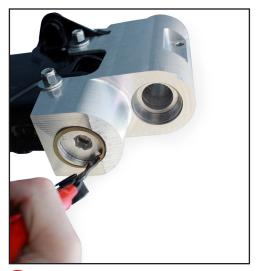
8 Install lower cir clip over lower set screw. Eenly tighten the top and bottom set screw untill seated at 60-70ft.
