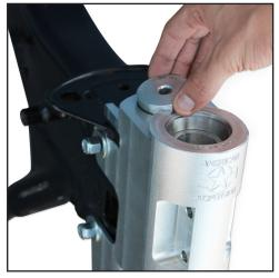
**5** Starting at the top, install top set screw (apply some anti-seize) - Do not fully tighten at this point.
