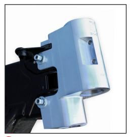
**9** Tighten cross bolts to 35ft lbs. Neck is now installed.
