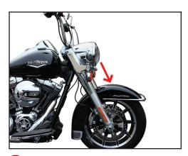
Install wheel and fender. Tighten axel and all bolts. Next loosen Axel and all bolts & fasteners except the top tree bolts. Bounce the bike using the brakes to rock the bike, so that the front end is fully seated. Now tighten the lower tree bolts and loosen the top tree bolts. Bounce the bike a second time. Now tighten all bolts and fasteners to correct torque and check for play in steering.
