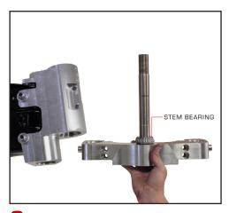
2 Pack supplied bearings with high quality bearing grease. Install 1 bearing on neck stem.
