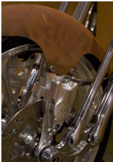
The D66 springer has a special springer P-26 brake caliper
