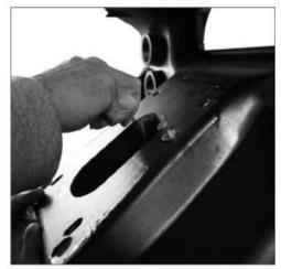
**6** Attach inner fairing to the front of the mount and tighten bolts.
