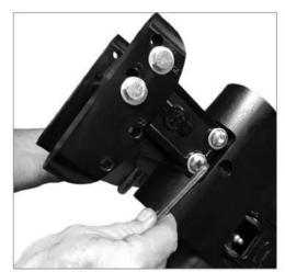
**5** Torque with 3/8" allen wrench and socket to 25ft.-lbs.
