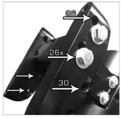
**4** Adjust the fairing mount wing bolts based on your wheel size (26", 26x", 30"). 26X is the most common fitment for 26" wheels
