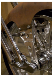
The D66 springer has a special springer fender bracket
