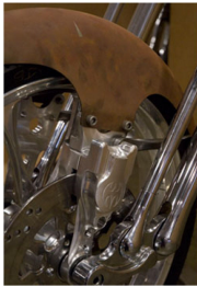
The D66 springer has a special springer P-26 brake caliper
