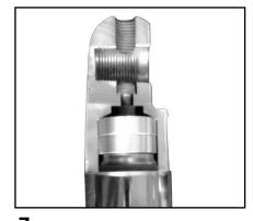
7 Check clearance between fender and lower tree. Install one or two top out spacers as needed in lower legs for fender clearance and use the provided limiters if needed, must use 2 per side on 2014
