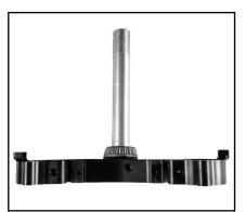
**2** Pack supplied bearing with high quality grease. Install stem into lower tree then install greased bearing on stem.
