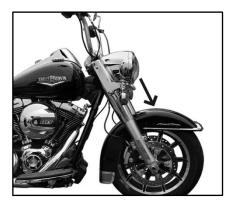
**8** Install wheel and fender. Tighten axle and all bolts. Loosen axle and all bolts & fasteners except top tree bolts. Bounce the bike a few times. Now tighten all bolts & fasteners to correct torque and check for play in steering. Install brake line to fit your needs. Reinstall removed parts to H-D specifications.
