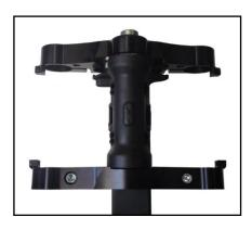
**4** Insert lower tree and stem into steering neck. Screw stem into top tree.
