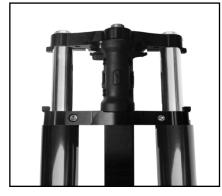
**5** Install fork cans on lower tree. Install both legs and torque lower tree bolts. Leave all top pinch bolts loose. Tighten stem while moving fork assembly until clicking disappears. Tighten 1/4 turn more. Trees should fall left & right with no drag. Lift legs up and down to check for any play in steering bearings.
