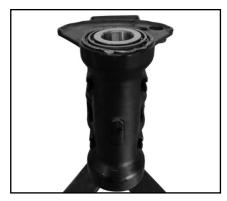
**3** For 2013 models and down re-use original upper bearing, while 2014 models and up, use provided bearing.
