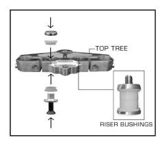
**1** Install riser bushing sets into top tree. Insert steering stop screws on the bottom of top tree.
