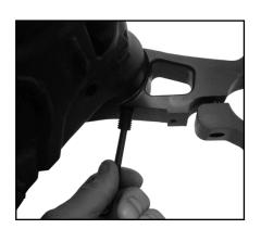
**6** Torque top tree pinch bolts. Then install stem pinch bolt on lower tree. Tighten all three pinch bolts to hold stem.
