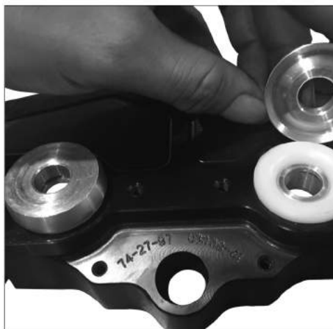
8 Place handlebar bushing caps into Delrin.
