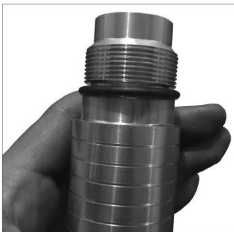
2 Insert o-rings into fork extensions.
