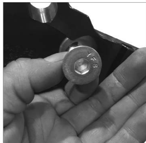
9 Insert 1/2-13 counter sunk bolt through the handlebar bushings.
