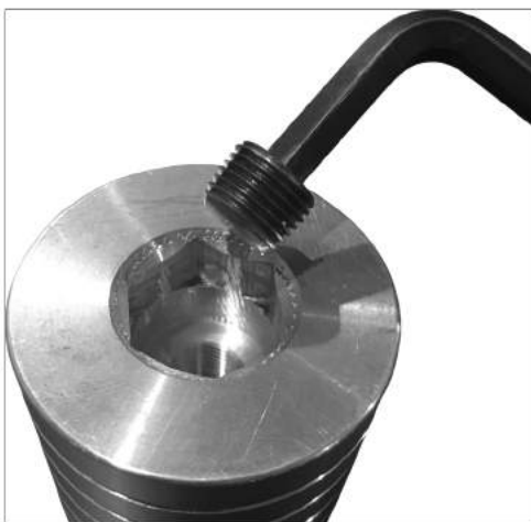
1 Install air plug into fork extensions.
